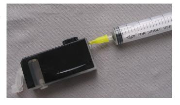
Step 5. Insert the syringe and needle and slowly inject the ink with the cartridge tilted so that the tank side is the lowest point.
