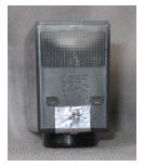
COMPLETELY BLACK CARTRIDGES: Fill until the syringe is empty. If bubbles start forming at the outlet during filling before the ink is finsihed, stop and let it dissipate and continue filling very slowly. If it continues to do this, stop injecting ink as the cartridge is now full.
